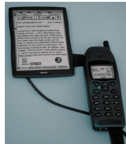
Sample image of electronic paper External monitor for mobile phone ©E Ink
