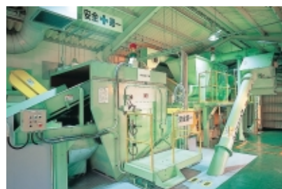
RPF (Refuse Paper and Plastic Fuel) equipment: facility for recycled solid fuel derived from wastepaper and waste plastics
