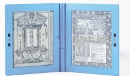
Prototype of E Ink Electronic paper (Cooperation: E Ink Corporation, Koninklijke Philips Electronics N.V., and Printing Museum, Tokyo)
