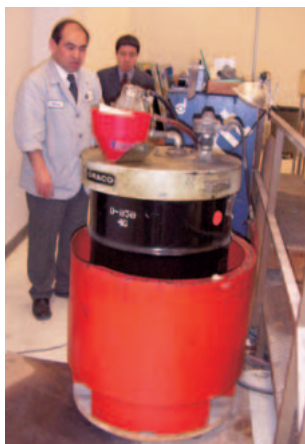
A metal drum is placed inside a special polythene container to prevent spillage while transferring waste ink (Toppan Interamerica Inc.)
