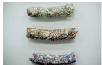
Through the RPF (Refuse Paper and Plastic Fuel) system introduced in 1999, waste plastic and paper is recycled as solid fuel. (Sagamihara plant)
