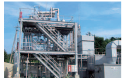
Cyclic use of VOCs in emitted gas as recycled solvents through reclamation and purification of emitted gases with solvent recovery processing equipment. (Matsuzaka plant)
