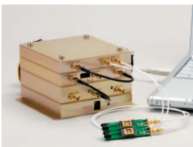
The ball SAW device won the Device Award at the Organic Materials Technology Exhibition held in July 2005 at the Tokyo Big Site. Its development of leading-edge material and application technology received wide acclaim. Exploiting the characteristics of high frequency oscillation that circles several hundred times around the surface of a crystal ball of 1mm in diameter, the device detects changes in extremely minute physical properties by amplifying them. One of its important features is that, by changing the sensitivity film, the sensor can perform different functions and integrate them. (The photo is the driving kit of the ball SAW sensor.)
