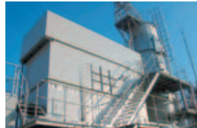
Equipment for recovering solvents from VOC effluent gas (Gunma Plant)
