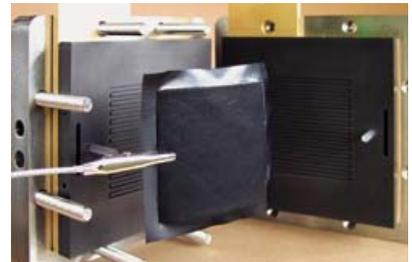
Membrane electrode assembly (the sheet shown at the center of the photo)
