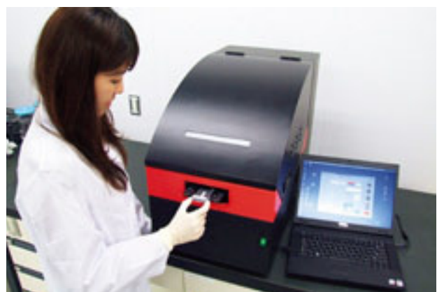
Genotype analysis system with SNP chips
