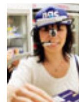
Eye-tracking camera for analyzing consumer gaze behavior
